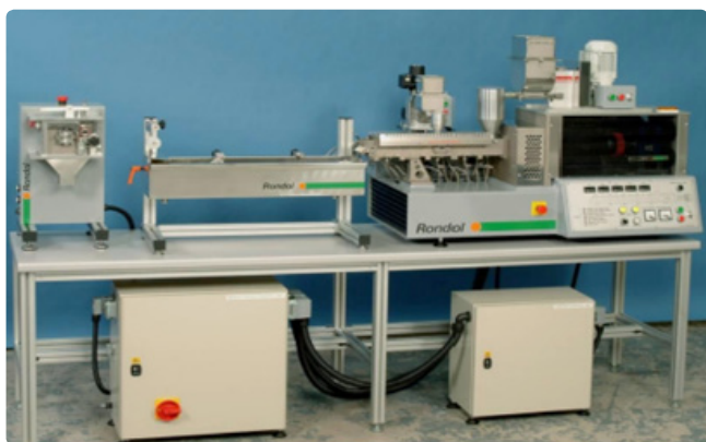
Figure 1: Extruder for thermoplastic compounding Pilot Line available at CeNTI facilities
