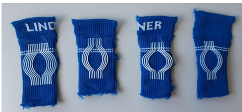
Strain-stiffening structures: 3D-printed at Heidelberg University
