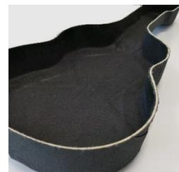
Picture 1: Defined fibre accumulations for semi-finished products from natural fibre nonwovens
