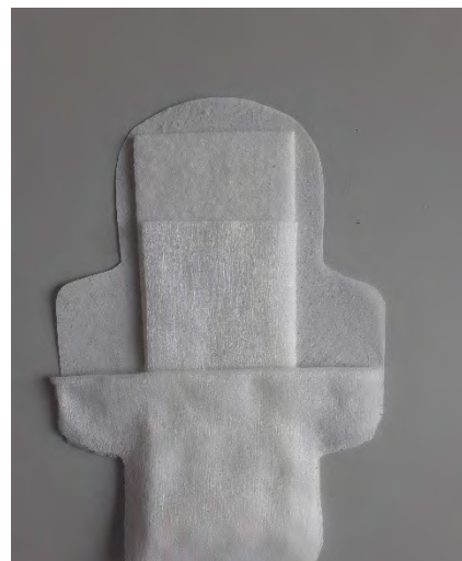
Figure 1: Nonwoven construction developed at STFI paves the way to reusable use for bio-based hygiene products | Picture: STFI
