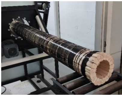
CF-reinforcement against restoring forces
