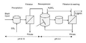
In brief, carbon dioxide is added to the black liquor which causes kraft lignin to be precipitated. The lignin is then filtered, resuspended in sulphuric acid, filtered again and washed to obtain a fuel purity grade lignin. The advantage compared to previous technologies is that the lignin have a low carbohydrate content (<3%) and very low ash content (0.5-1%).
