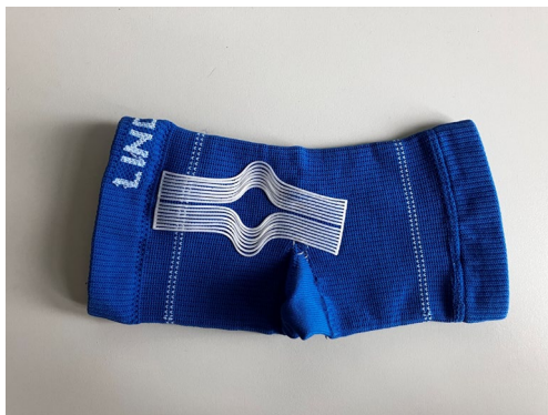
Ankle bandage with 3D-printed strain-stiffening structure
