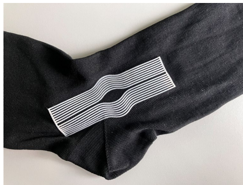
Stocking with 3D-printed strain-stiffening structure
