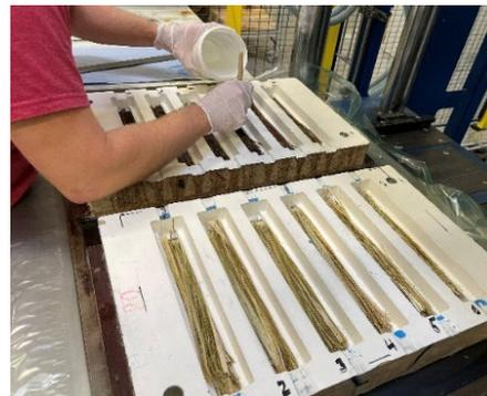
Production of fibre composite samples with bast fibre reinforcement
