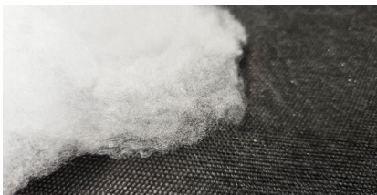
Crimped filaments made of PLA/BioPE
