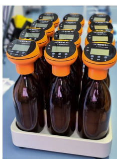
Testing of biodegradability using the OxiTop®-IDS BOD measuring system
