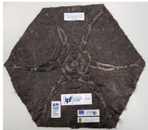
Fig. 4: Lightweight stool on 100 % rCF-nonwoven
