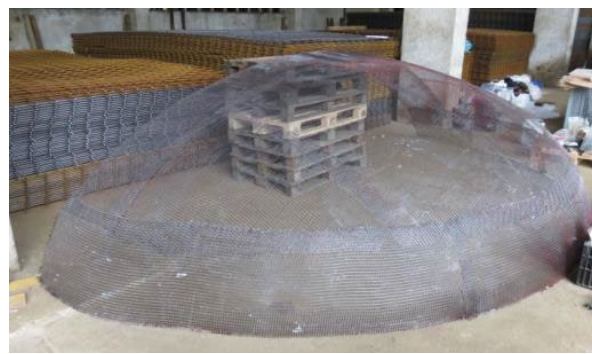
Fig. 2: Filigree reinforcement made of carbon fibers
