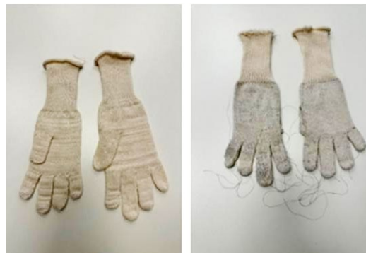
Gloves made from 100 % MAC/CO yarn (left) and from MAC/CO yarn + covering yarn made from Shieldex® yarn + MAC/CO yarn (right)
