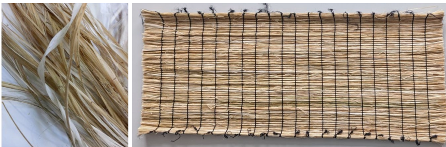
Hemp bast bark (left) and warp knitted fabric made from endless hemp bast strands using KEMAFIL® technology (right)
