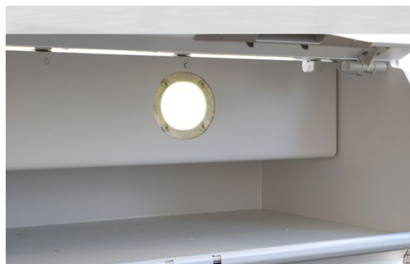
Substitution of the hinges of a luggage compartment with flexible fibre-reinforced plastics (© Wingdesign)
