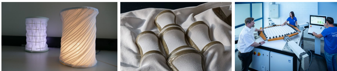
Lampshades developed in the project (left), sample of pre-stretched textile (centre) after being processed on a stenter frame (right; © STFI/Dirk Hanus)
