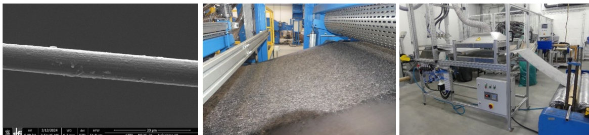
SEM image of a resized carbon fibre (left), production of nonwovens from carbon fibres (centre) and test stand for resizing nonwovens from carbon fibres (right)
