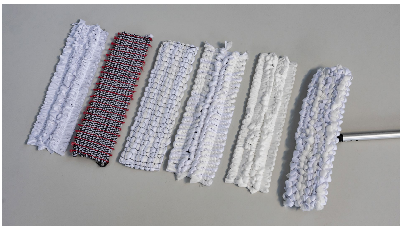
From the selvedge strip via the KEMAFIL® strand to the surface (Photo: STFI / Dirk Hanus)
