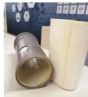
Tube liner resined and UV cured in a damaged sewer pipe (left), assembled (right)
