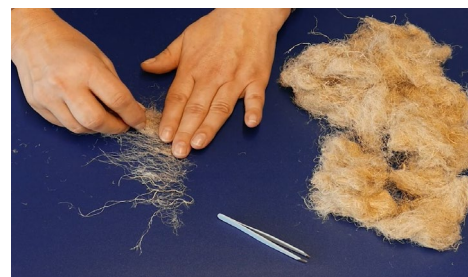
Manual preparation of a fibre sample
