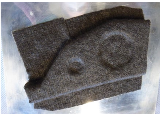
Fig. 2 Part of a C-pillar from the automotive sector of Alpha Sigma GmbH, left: Preform (nonwoven made of basalt and carbon fibers) draped in the mold, right: nonwoven-based composite (after impregnation with bio-based epoxy resin in a vacuum infusion process).
