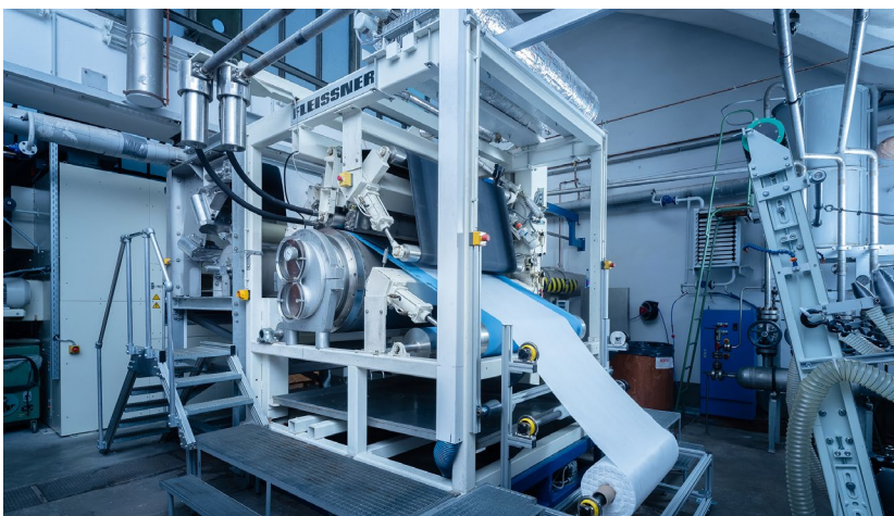
Spunlace line for the production of spunlace nonwovens at STFI
