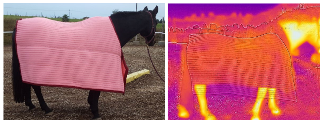
Sweat rug in practical test: real image (left), the infrared image shows evaporative cooling (right)
