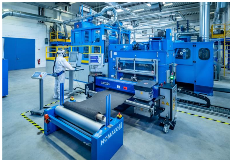
Carbon fibre pilot plant at STFI: Production of mixed fibre nonwovens
