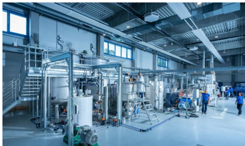
Wet fleece technology center at STFI: Production of short fiber nonwovens
