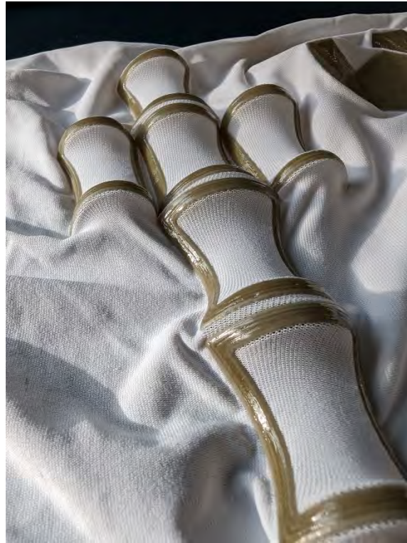
Figure 2 - Sample of a pre-stretched textile printed with WEVOPUR 71/25 MT/3 /WEVONAT 300 (Copyright: STFI)
