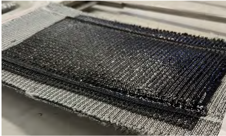
Figure 1: Functional sample of a sandwich-structured surface element, coated with a Wevopur potting compound (Copyright: STFI)
