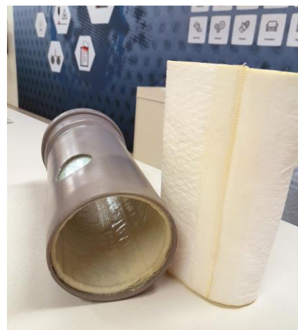
Tube liner made-up (right) and resined as well as UV cured in a damaged sewer pipe (left)
