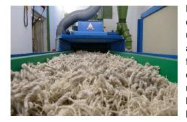
Most of the reclaimed fibres produced in Germany are processed in the nonwovens production. These nonwovens are used for instance in vehicle construction, in general machine and device construction as well as in the home textile and furniture industry. The nonwoven can be formed from reclaimed fibres by carding or aerodynamically by forming a randomized web. The consolidation of the web can be done by needl-punching, by water jets, in a thermofusion oven or by stitch-bonding technology.
