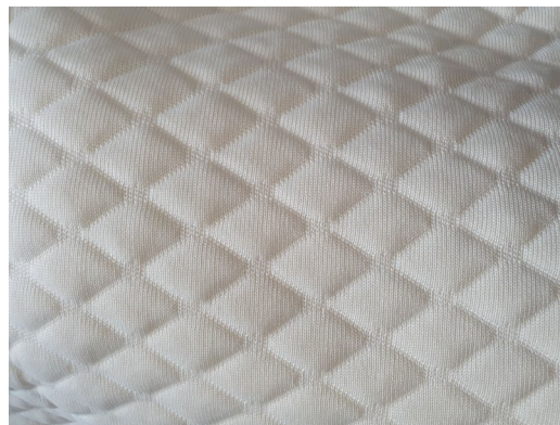
Double-layer knit with internal filling threads for use as a patient coverage
