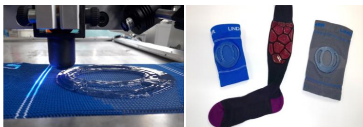
3D printing with simultaneous UV curing (l.), project demonstrators (r.)
