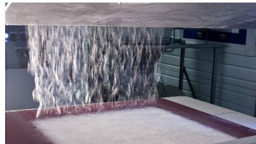
Production of a meltblown layer at the STFI
