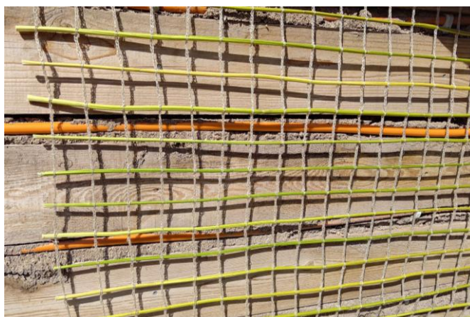
Prototype of a plaster-bearing lattice made from hemp stalks
