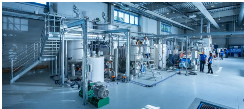
Pilot-Nassvliesanlage am STFI (Foto: ©Hanus/STFI)
