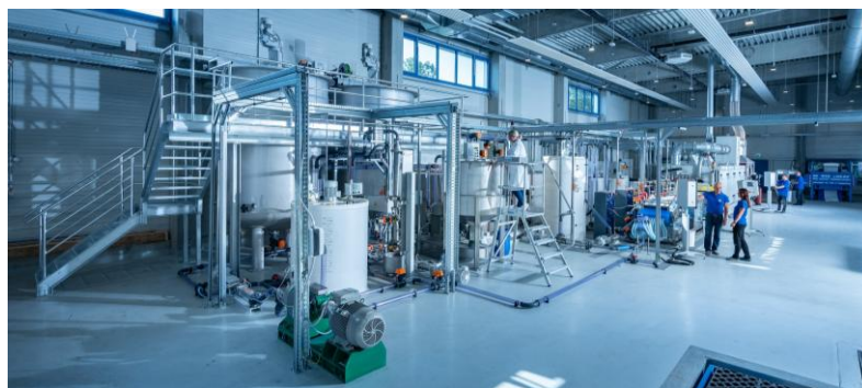
Pilot scaled Wetlaid line at STFI (Foto: ©Hanus/STFI)
