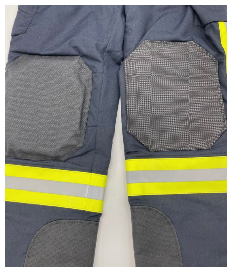
Firefighter's trousers: Benchmark on the left – SeFiPro on the right
