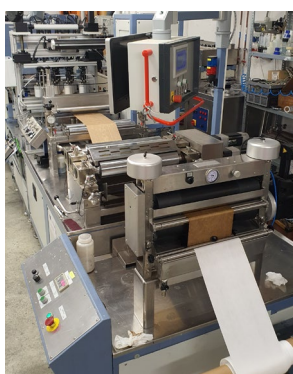
Functionalisation of meltblown nonwovens by dip coating and drying filter layer
