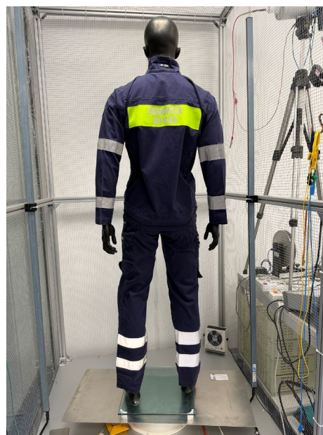
Test rig (partial view) with the STFI electrostatic human model for testing the charge-transfer electrode system
