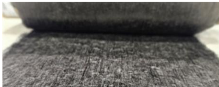
rCF tape for fibre-reinforced composite applications
